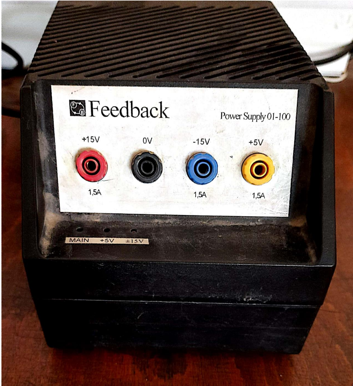
DC Power supply Input : 220 V AC Output : +5 V, +/- 15 V DC Model Feedback Power Supply 01-100
