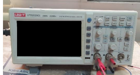
Digital storage oscilloscope Bandwidth : 25 MHz Sample rate : 250 MS/s Mains voltage input : 100 - 240 V AC Mains frequency : 50/60 Hz Model : UTD 2025 CL
