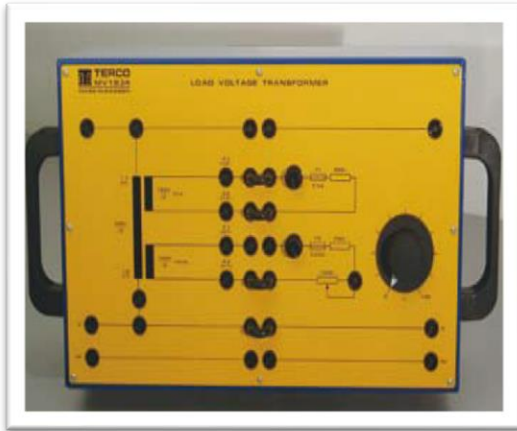
Voltage Transformer with load combinations combinations Model TERCO MV 1934
