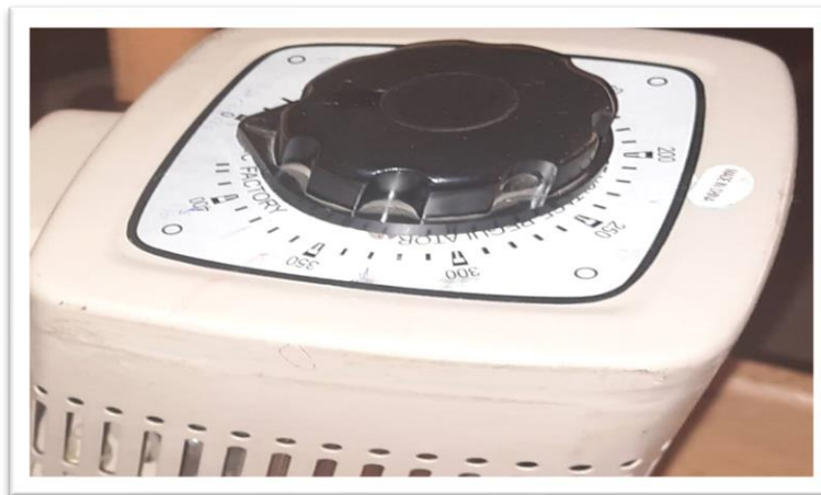
Voltage Regulation Auto transformer Input Voltage : 380VAC Output Voltage : 0-450VAC
