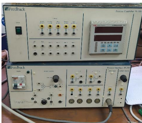
Process Controller (top) with Process Interface Process Controller model : 38-300 Process Interface model : 38-200
